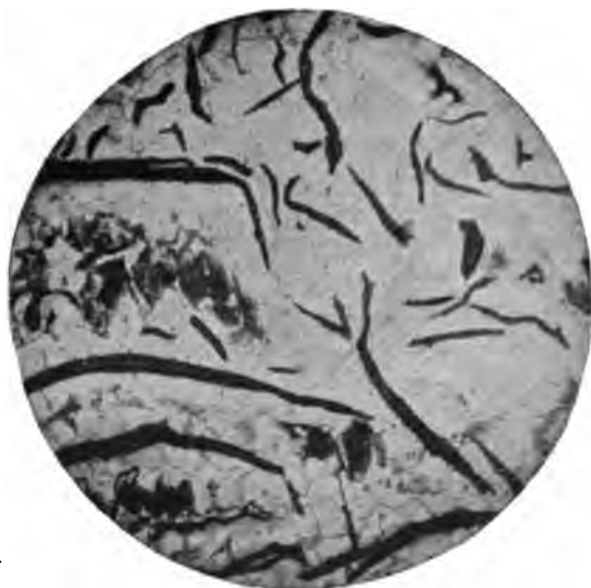
FIG. 178.—Gray Cast Iron. Magnified 100 Diameters. (Boylston.)
